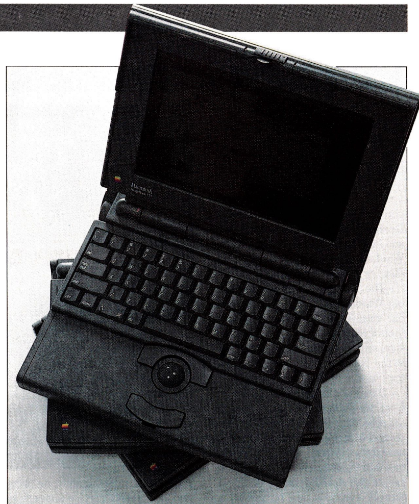
The 140 is equipped with four megabytes of RAM and a 20 megabyte hard disk
